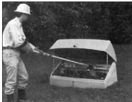
Figure 3. Hinged top provides unobstructed access.
